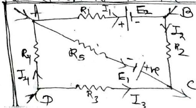
Explanation:- In the given closed circuit ABCD,  $R_1, R_2, R_3, R_4, R_5$  are the resistances &  $I_1, I_2, I_3, I_4, I_5$  are the currents in the five arms of the circuit, with two e.m.f sources  $E_1$  &  $E_2$ .
