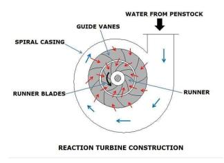
Reaction turbines are the type of turbine that formulates torque by countering the pressure or mass of a vapour or liquid. It utilizes the pressure as well as the momentum of the striding liquid to fluctuate.
