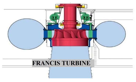
Francis turbine is used for the production of abundant electricity often in medium or largescale hydropower locations. In the Francis turbine, the fluid enters these turbines radially implying that it enters the turbine perpendicular to the rotational axis.
