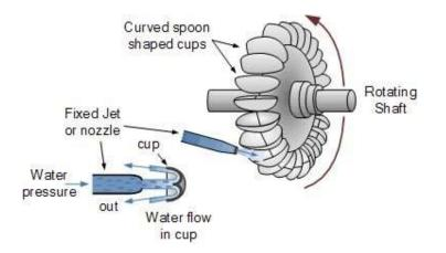
In the case of an impulse turbine, the working principle revolves around two main factors: the mass of the flowing water or fluid and the change in velocity of the flow as it enters the turbine and exits after impact.
