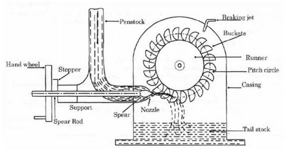
The impulse turbine comprises several essential components that collaborate synergistically to facilitate the conversion of the kinetic energy of a high-velocity fluid jet into mechanical work. These components include the runner, buckets, nozzle, spear, casing, penstock, and potentially a braking jet.
