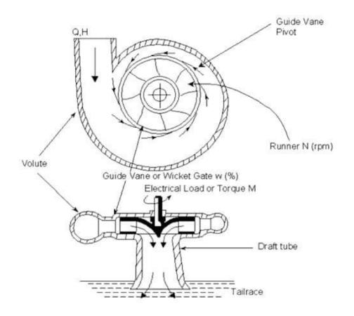
The working principle of the reaction turbine is based on Newton third law of motion. The water enters into the spiral casing with high velocity and low heads.
