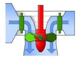
The propeller-type turbine is a type of turbine in which the flow is inward with a runner shaped propeller it can be seen in ships and submarines and it is provided with either remedied or elastic blades.
