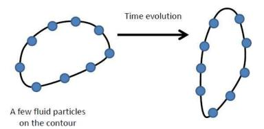
In the course of time, these fluid particles move about with the flow and thus the contour moves with them accordingly. We calculate the material derivative of the velocity circulation bounded by this contour:
