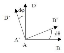
Again, this is easy to show that  $d\theta + d\varphi = (\partial v_y / \partial x - \partial v_x / \partial y) dt$ , or equivalently:
