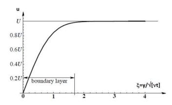
The region in which the velocity field departs significantly from the constant flow U is called boundary layer: according to the expression of u(y,t), this layer is proportional to  $\sqrt{vt}$ . Hence, for fixed time, the boundary layer decreases as  $1/\sqrt{Re}$ .
